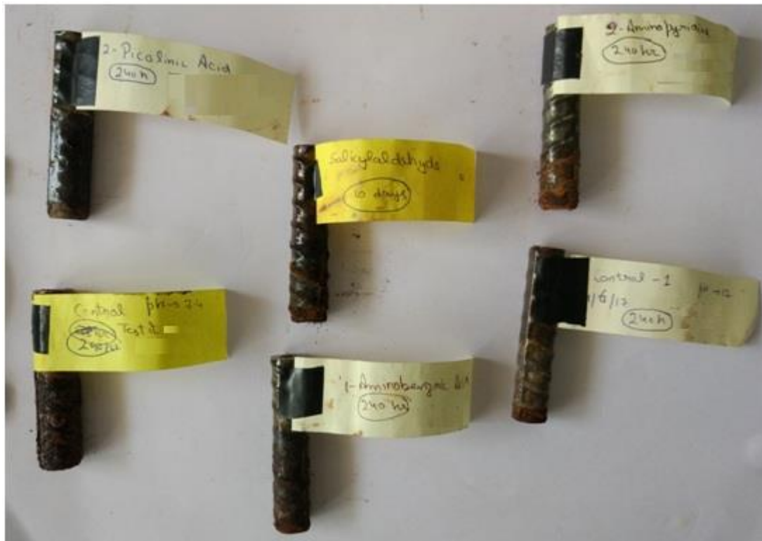
Figure 5.8: Steel specimens after measuring Half-cell Potential and Linear Polarization Resistance, immersed in different solutions after 240 hours
