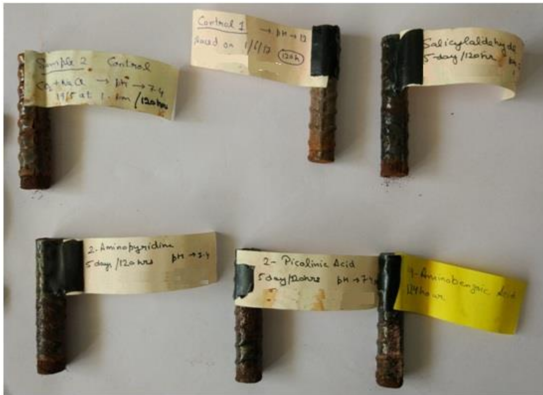
Figure 5.6: Steel specimens after measuring Half-cell Potential and Linear Polarization Resistance, immersed in different solutions after 120 hours
