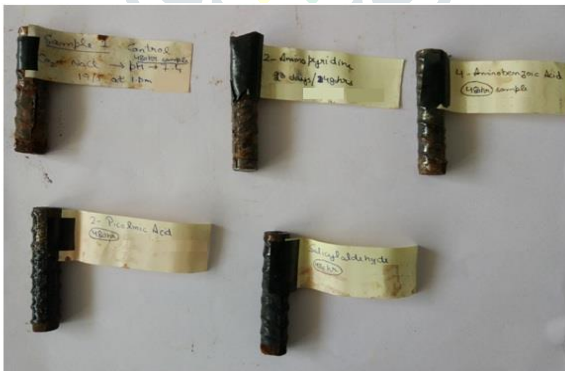
Figure 5.10: Steel specimens after measuring Half-cell Potential and Linear Polarization Resistance, immersed in different solutions after 480 hours
