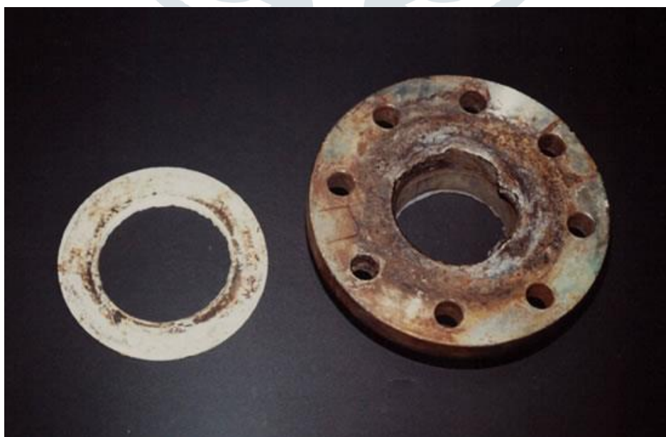
Figure 1.4: Crevice corrosion on a stainless steel flange
