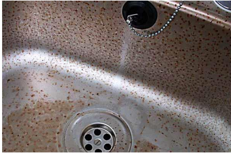
Figure 1.6: Pitting corrosion on sink surface (Source : http://www.amteccorrosion.co.uk )
