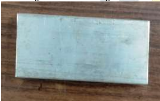
Fig.5. Aluminium Alloy 6082 before machining
