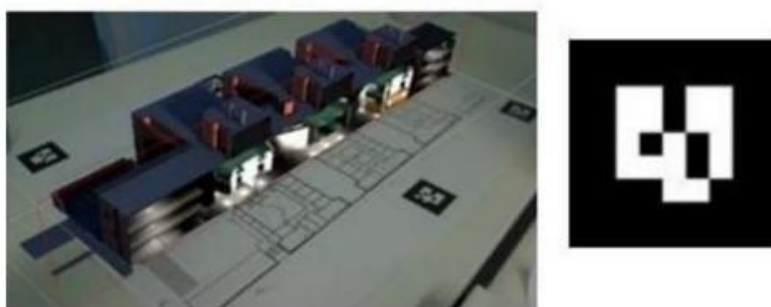
Fig 3.1 Superposition of the virtual and real scene using a 2D marker
