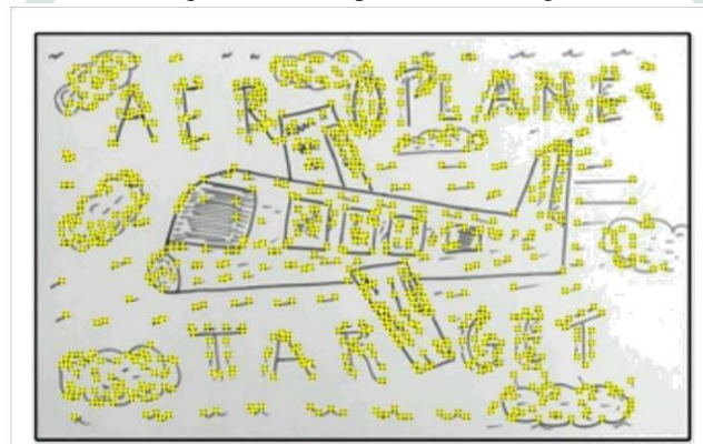
Fig 4.2 Feature Detection using Line Detection Algorithm of a 2D Aeroplane Asset/Target.
