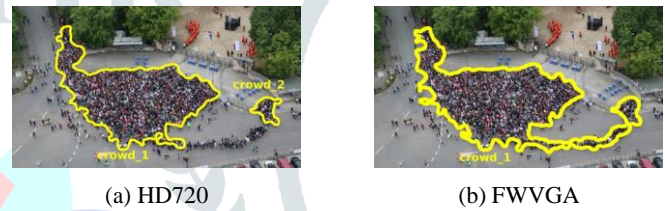
Fig. 5: Scaling slightly changes the crowd detection results because individuals may be connected to crowds.
