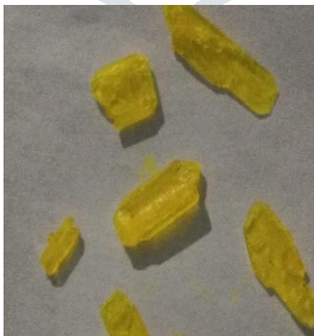
Fig 1: The grown sodium para-nitrophenolate dihydrate crystals
