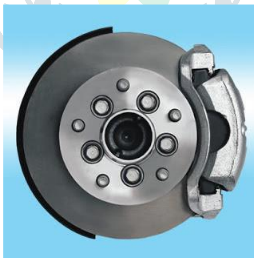
Fig.1 ventilated disc brake and assembly.
