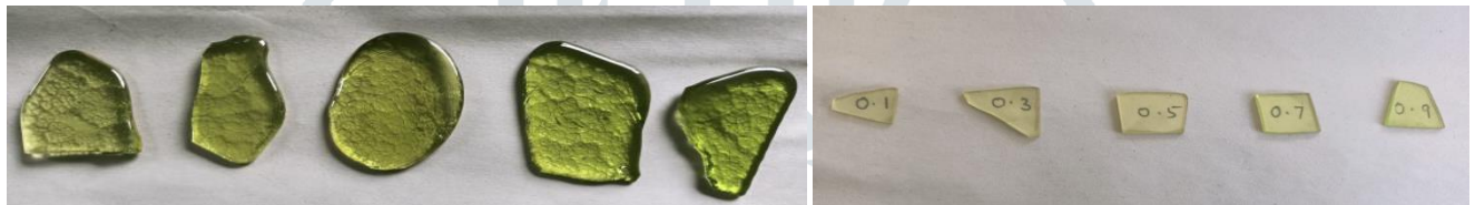
Fig.1. Fabrication of glass samples – ( Before & after polished )
