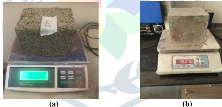
Fig. 4: Measurement of Weight of (a) Hempcrete & (b) Conventional Concrete Cubes
