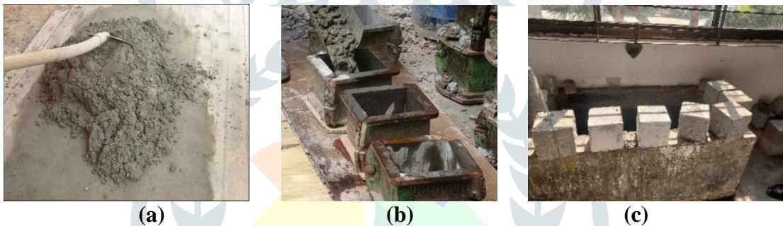
Fig. 2: (a) Mixing, (b) Molding & (c) Curing Of Concrete
