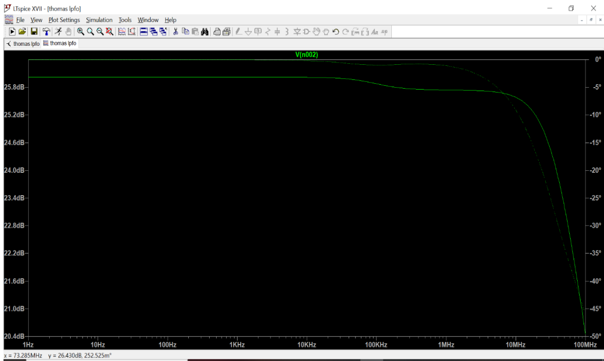
FIG. 10 SPICE SIMULATION OF APPROXIMATED FRACTIONAL CHEBYSHEV LOW PASS FILTER (ORDER N=1.1)
