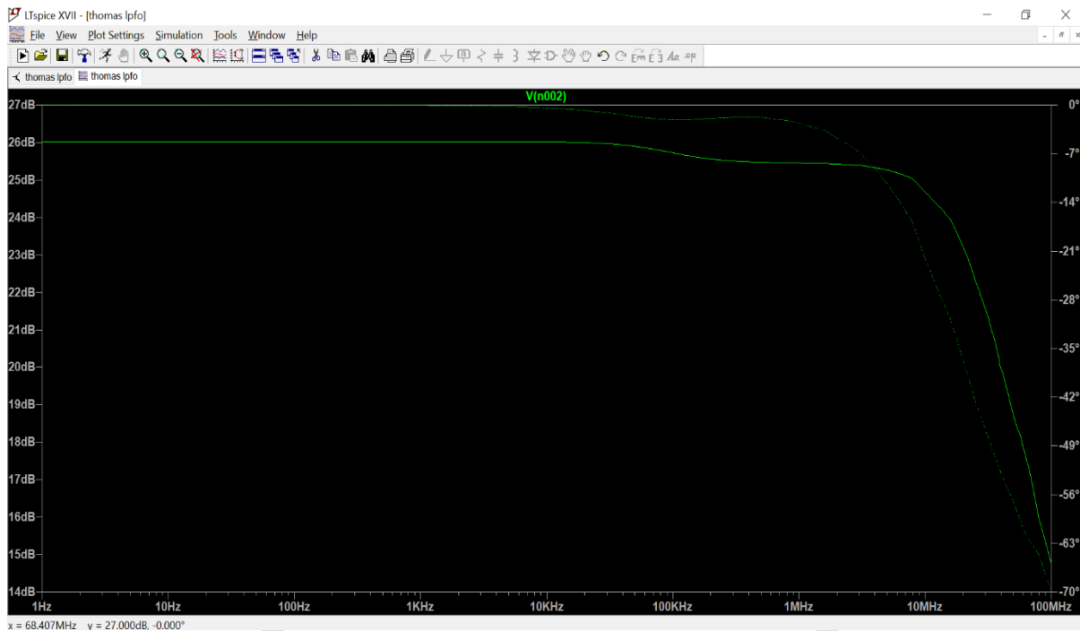
FIG. 12 SPICE SIMULATION OF APPROXIMATED FRACTIONAL CHEBYSHEV LOW PASS FILTER (ORDER N=1.5)
