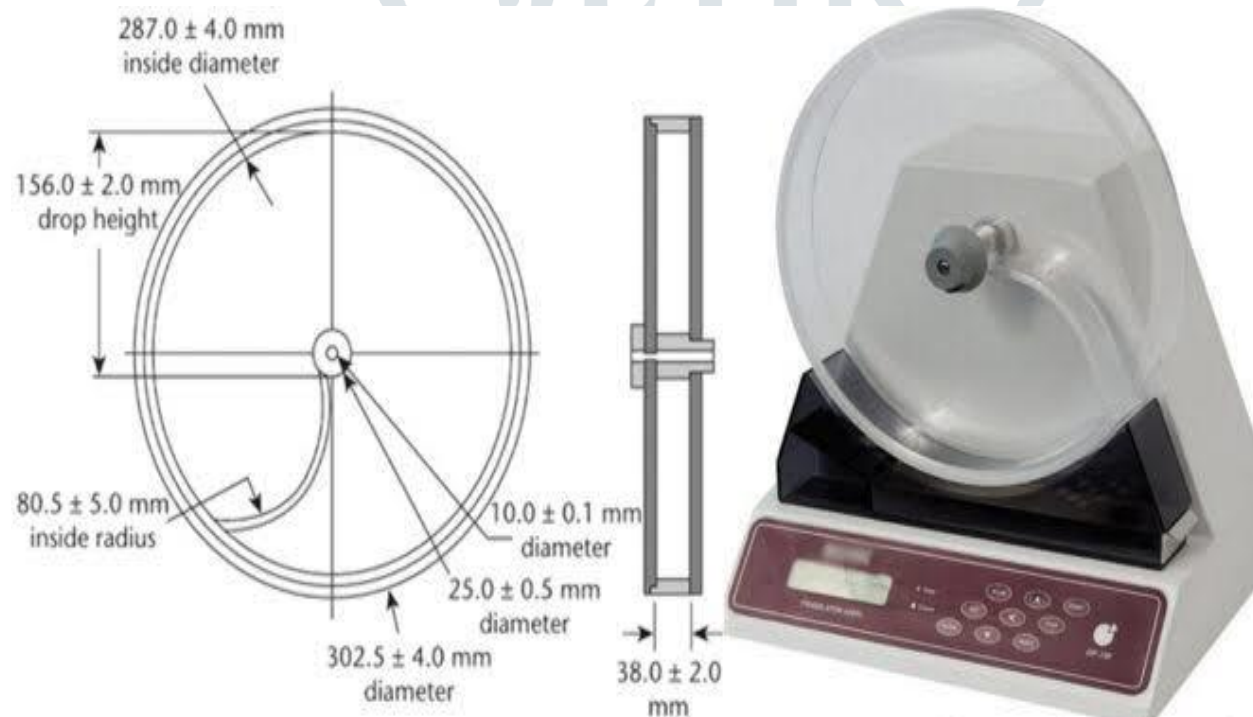
Fig: Roche Friabilator For Uncoated Tablets
