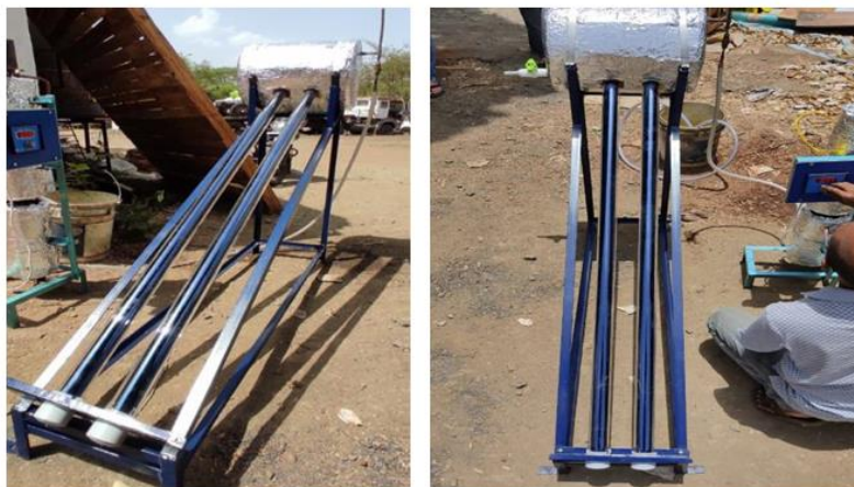
Figure: 4. Solar water heating section
