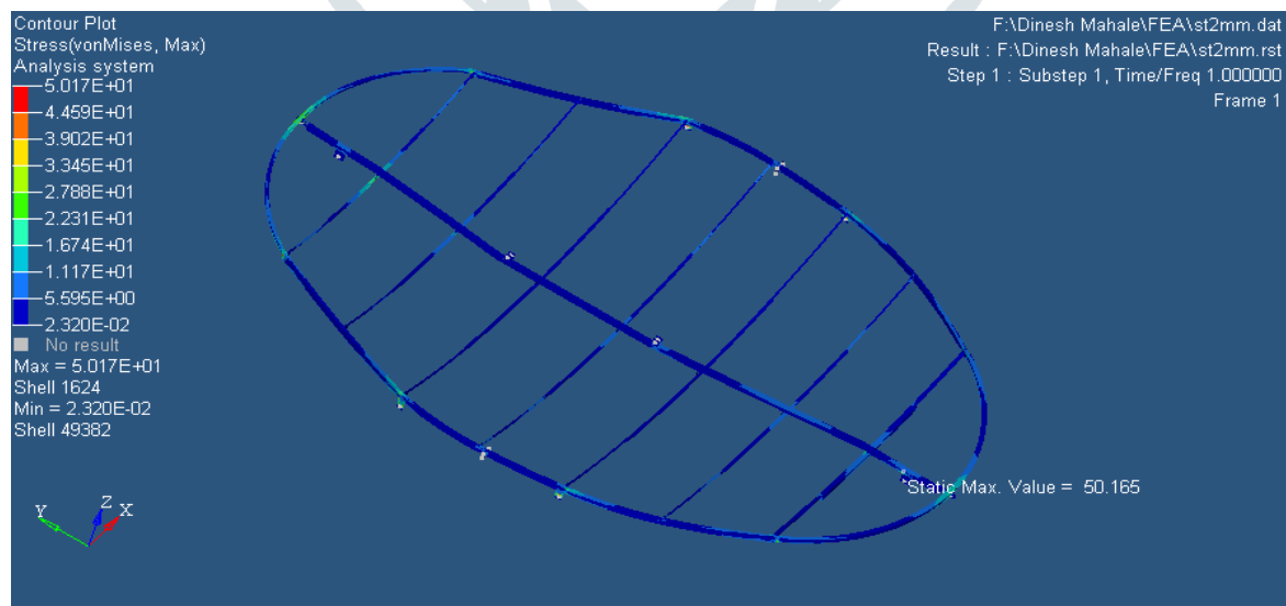
Fig. 3.8 Maximum stress – 2 mm thickness - Steel
