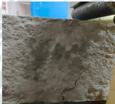
Fig. 5 Formation of cracks on prism under loading
