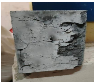
Fig. 1 Cube after applying load
