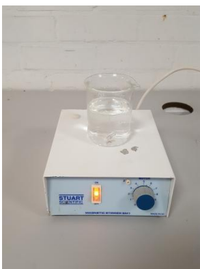
Fig 3.3: Magnetic stirrer with a beaker containing the sample and a magnetic stirrer.
