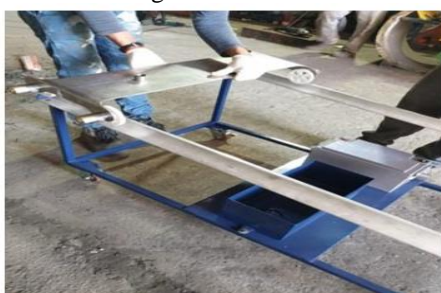
Figure 6: Installing the Cleaner that has Four DC Motors and Four Wheels on the Structure. Figure 7: Fitting the Solar Panel on Board. Figure 8: Final Sketch.
