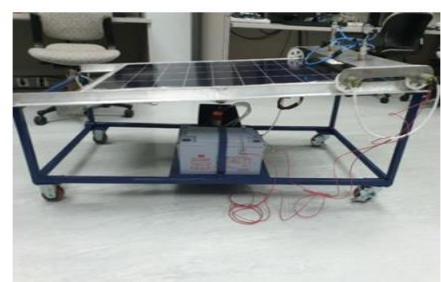
Figure 6: Installing the Cleaner that has Four DC Motors and Four Wheels on the Structure. Figure 7: Fitting the Solar Panel on Board. Figure 8: Final Sketch.
