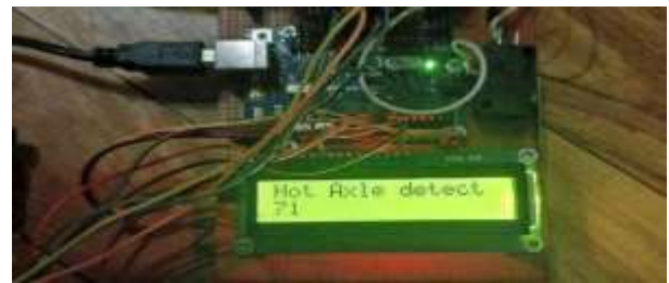
Figure No. 10 Hot Axle Detection
