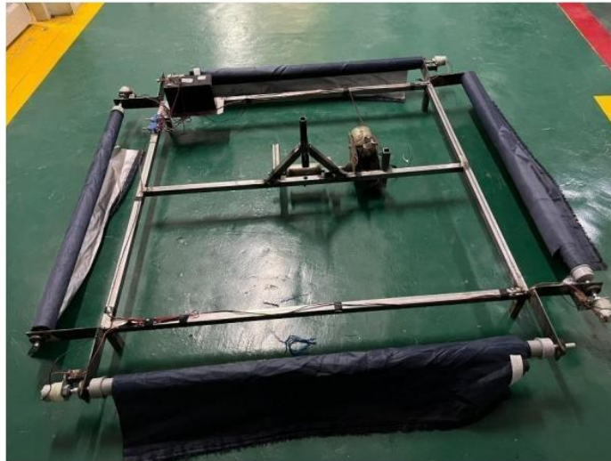
Fig 4.1 Fabricated Car Cover with side rollers and center attachment for Umbrella
