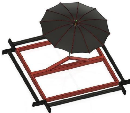
Fig 3.6 Isometric View of Automatic Car Cover with umbrella in open position
