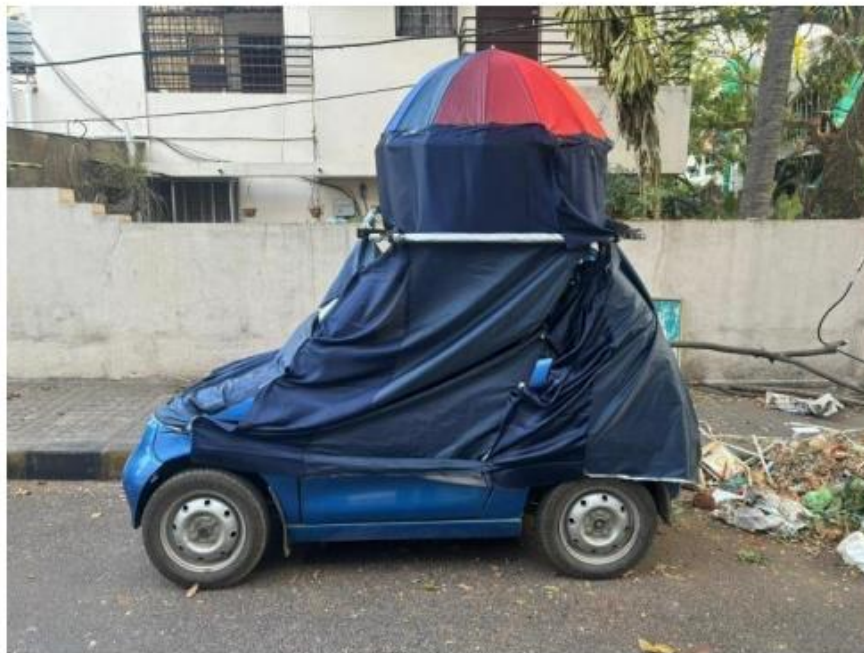
Fig 4.2 Fabricated Car Cover with fully opened mode
