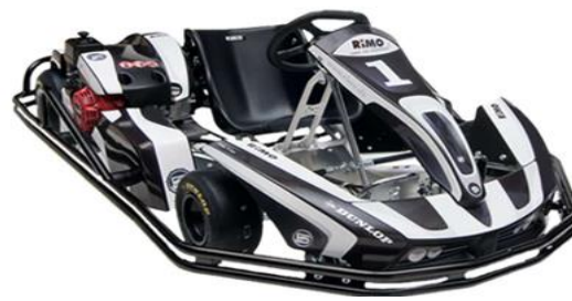
Figure 2. Go Kart with Chassis Designed to be Flexible.
