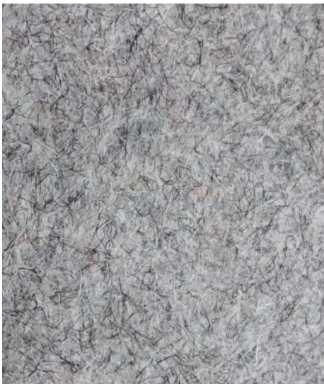
Fig 2 Nonwoven Mat made with Chicken Fibers
