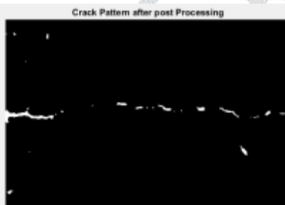
Fig25: Clean Crack Patter after Post Processing.
