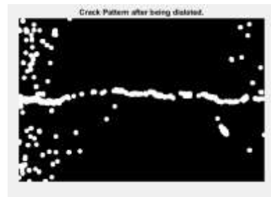
Fig22: Crack Pattern after being dilated.
